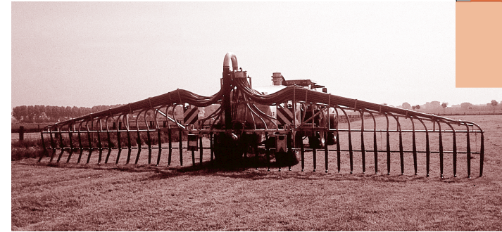
Figure 2 Band spreader fitted with rotary distributor to improve lateral distribution
